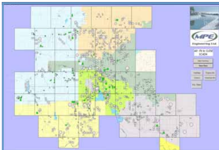
RAM overview screen showing each irrigation system in the WID. Sub screens show system usage, crop types and contract information. When a system is green, it means it is actively irrigating.
