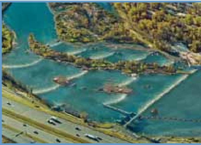
Once completed, the manmade "islands" will increase the upstream water level thus eliminating the "drowning machine" effect caused by the weir
